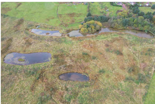
Aerial view of small flood storage ponds in upper catchment at Ruddenleys
