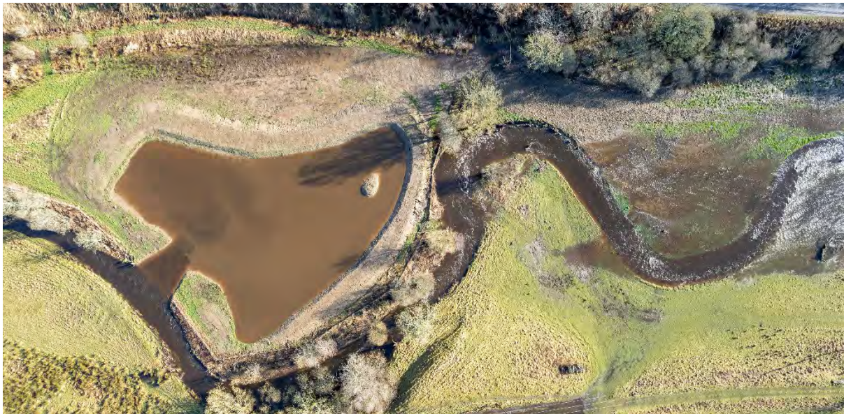
New flood storage pond and downstream meanders at Nether Kidston during high flow conditions.
