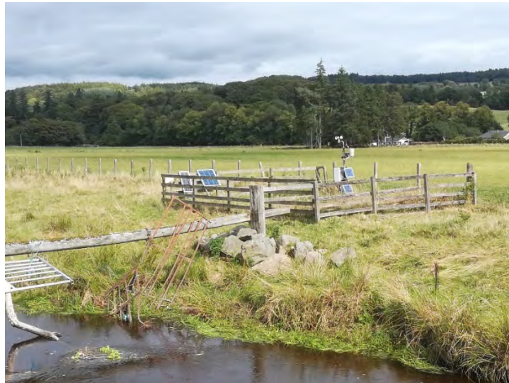
Main Automatic Weather Station at Darnhall – see Fig 7
